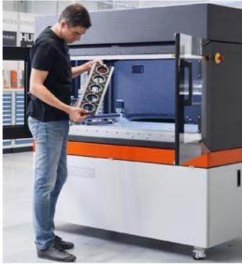
The STUDIO G2 has a unique dual extruder equipped with two 0.6 mm specialized nozzles made for printing with engineering-grade materials, including fiber reinforced, efficiently at high-resolution.
