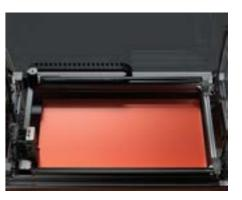
Preparation time is significantly reduced for all print projects by the fast-heating print bed. Capable of quickly reaching 100°C for optimal print bed adhesion with a variety of high-quality materials.
