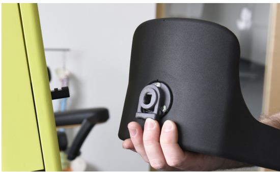
The quick release system of the neck support demonstrates the essence of laser sintering: The design of the two moveable parts printed inside each other would not be possible with either a conventional manufacturing system or any other affordable 3D printing process.
