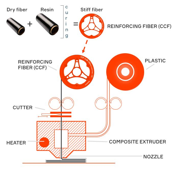
Reinforcing material is made with dry continuous fibers preliminary impregnated and then cured, providing a perfect material quality.
