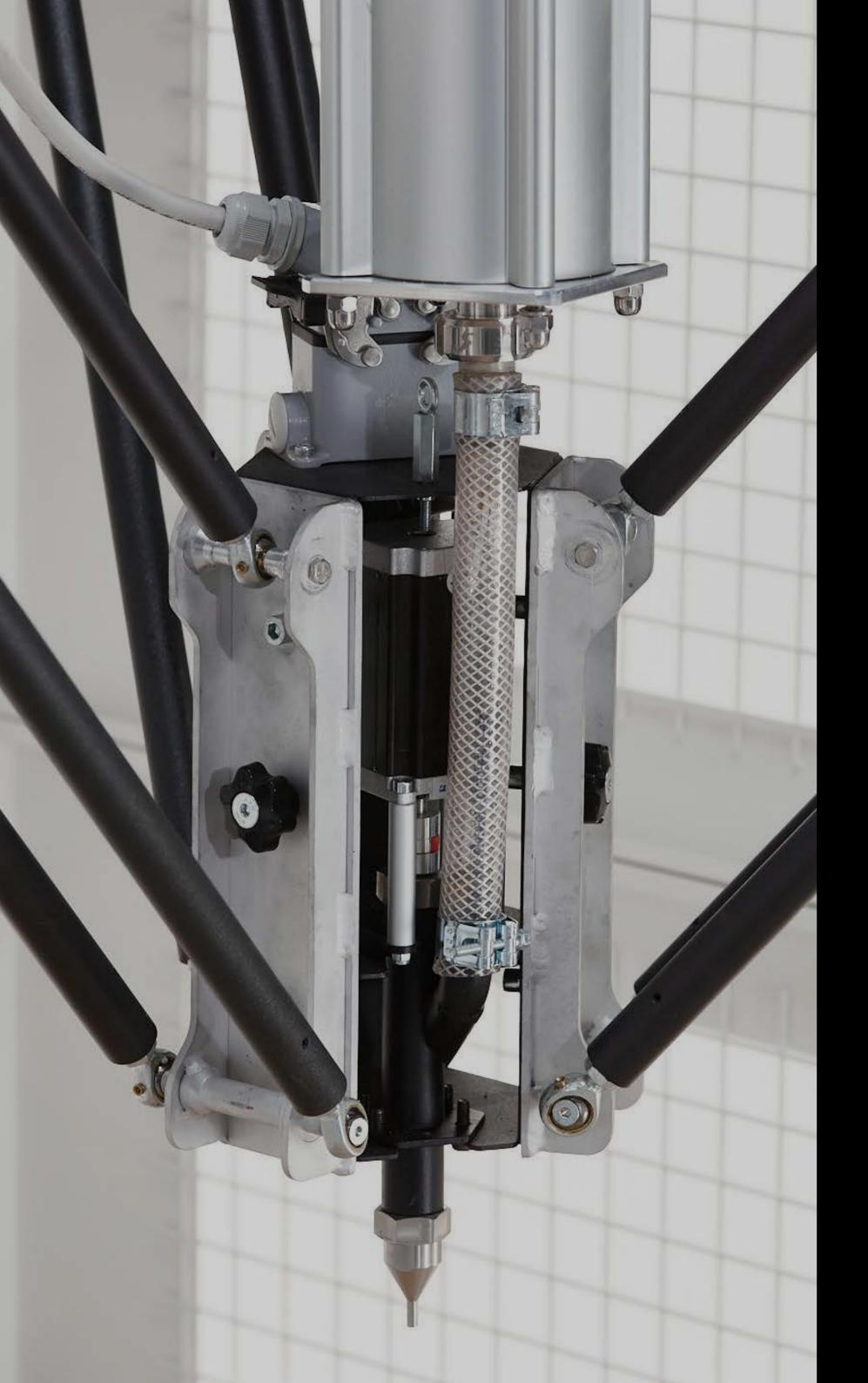
Delta WASP 3MT INDUSTRIAL 4.0 LDM is compatible with LDM WASP Extruder XL and allows printing clay materials in big size.
