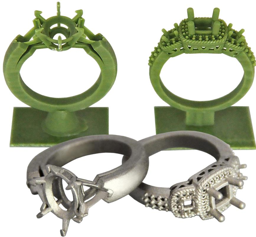
EnvisionTEC's innovative direct investment casting material, Easy-Cast EC3000 has three times more wax than any polymer based material, including EnvisionTEC's EC500 material.
