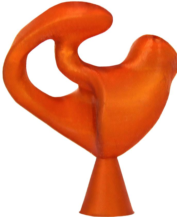
EnvisionTEC's E-Silicone material offers a solution to produce soft silicone otoplastics by the additive manufacture of cocoon molds. The custom fit E-Silicone molds may be injected with medical-grade silicone materials. The eggshell-like mold may then be easily broken away, leaving a soft, flexible shell. These shells can provide patients with increased comfort, better retention, better acoustic seal, more gain before feedback and improved sound quality.
